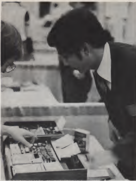
Janson Chang of Enerton, Inc. (2726 Middleborough Circle, San Jose CA 95132), explains his PA-EDU80 Z-80 based microprocessor trainer and self-learning set. The unit has an on-board 1K read-only memory monitor, a solderless breadboard area and a 36-key keypad. Prices start at $195 for the computer board only.
